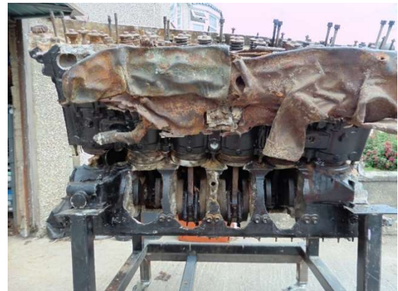
Starboard Side, showing impact damage, (engine partly dismantled for restoration)
